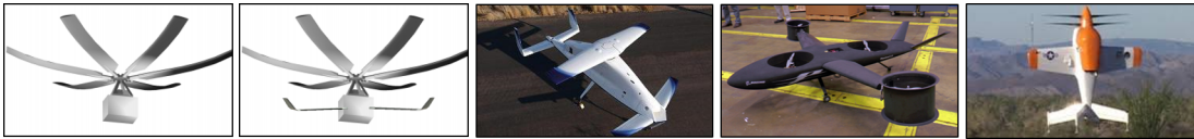
FIGURE 4.3: (a) AAD (b) Lift-compound AAD (c) Stopped Rotor (d) Fan-in-body/Fan-in-wing, and (e) Tailsitter were chosen as the top five vehicle configurations.
