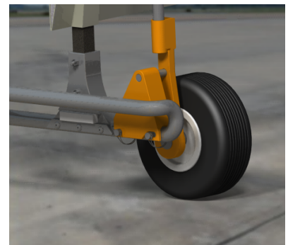
FIGURE 3.4: Dual-mode landing gear.
